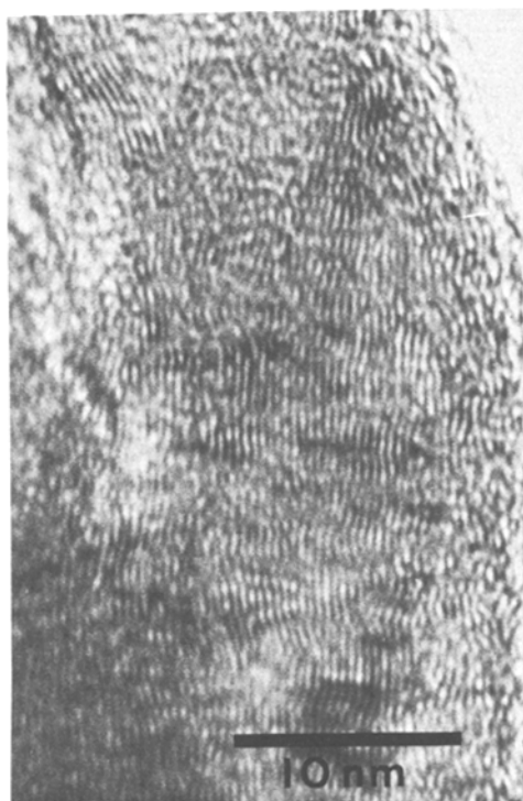
Figure 3 Extensive lattices induced by bromine treatment ( \Delta f + 49 nm).
